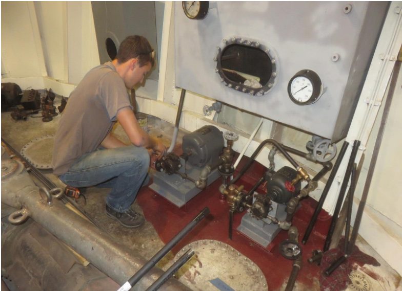
Barry Witte's students continue to make progress on the smoke screen generator replication.
