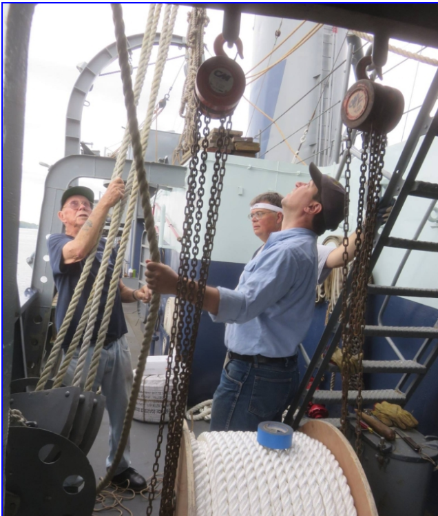
Rigging the boat falls with the new line donated by Les Catharine.
