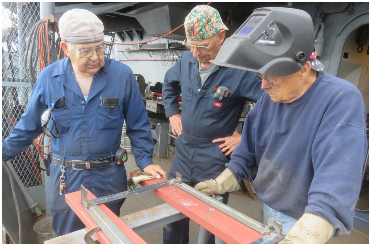
Our welding team of Doug Tanner, Tim Benner and Dave Mardon fabricating a cover for the B-3 vent space.
