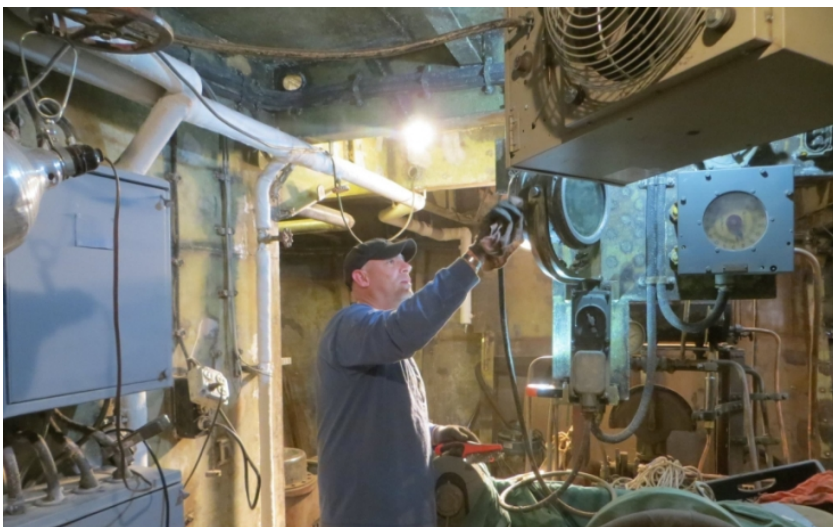
Nate Shakerley prepping the aft steering gyro repeater for restoration.
