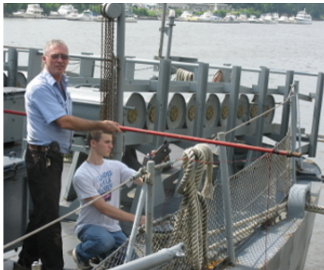
Gary Sheedy improvising with a 10' applicator to take cathodic protection readings.
