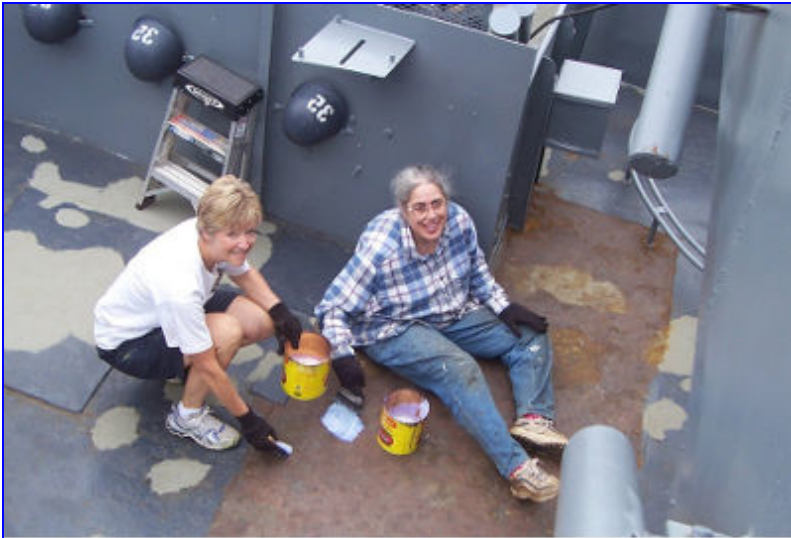
Jan Sweiger and Robin Larner getting ready to apply Corro Seal.
