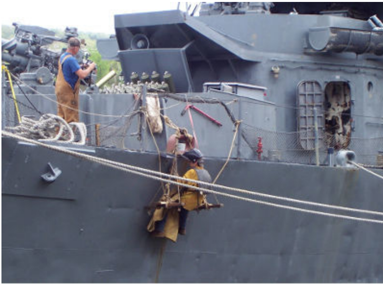
Laird and Brandon welding down chocks.
