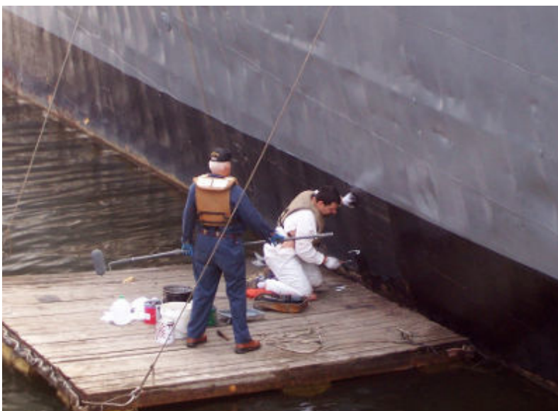
Brandon Easley and Joe Delfoe repainting the port boottop.
