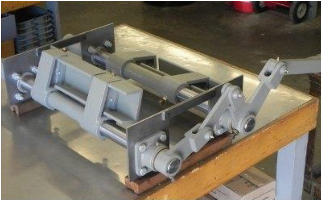
The new depth charge release mechanism fabricated by George Christophersen.
