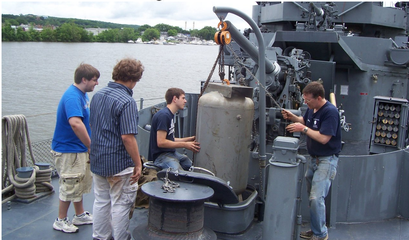
Barry Witte and his crew relocate the forward LP Air Compressor.
