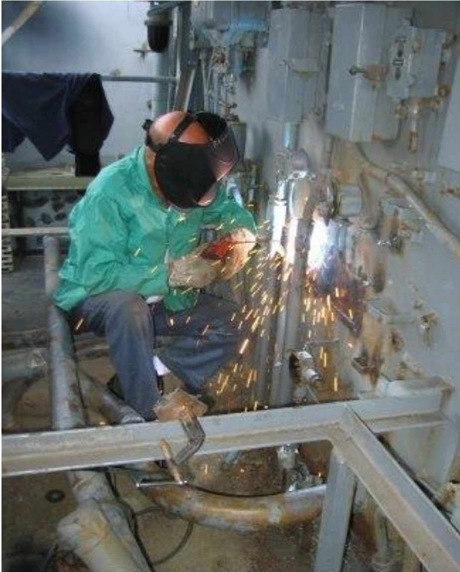
You can tell by the shiny head that it's Ben- ner welding a patch on the flying bridge.
