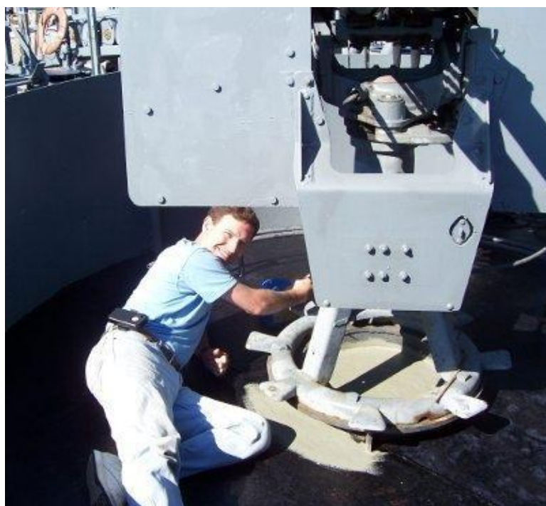
Rob Haley, SLATER volunteer and sometimes airline pilot, applies primer to an aft 20mm gun tub deck.
