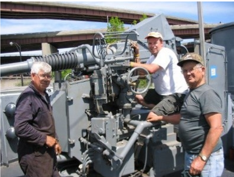
Butch Warrender, Scott McFadden and Laird Confer put the elevation gear back together on gun 42.
