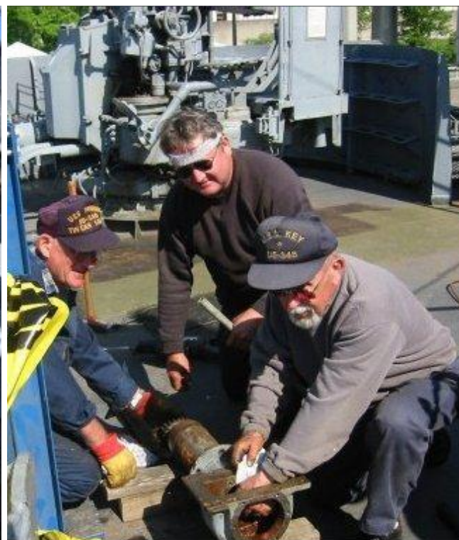
The 40mm gun gang Pete Houle, Doug Strieter and Stan Suzdak working on the elevation gear.
