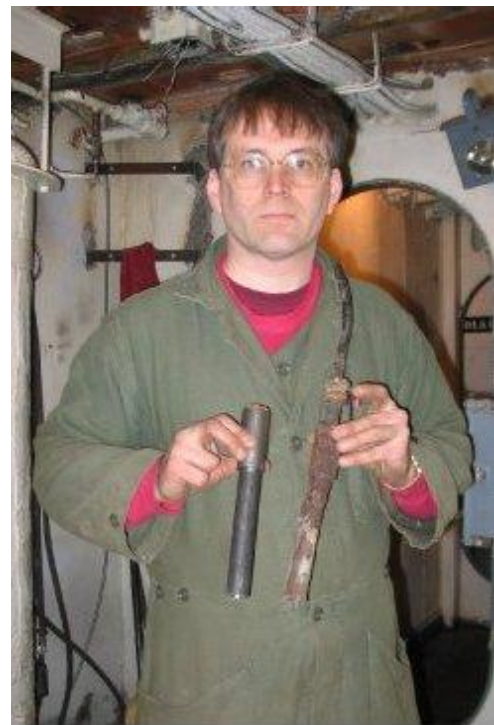
New stuffing tube, old stuffing tube. Note the difference!
