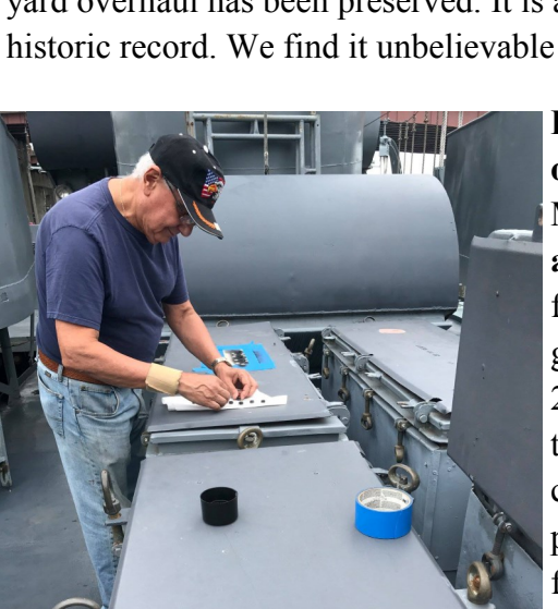
Vic Consiglio stenciling the 20mm ready service lockers.
