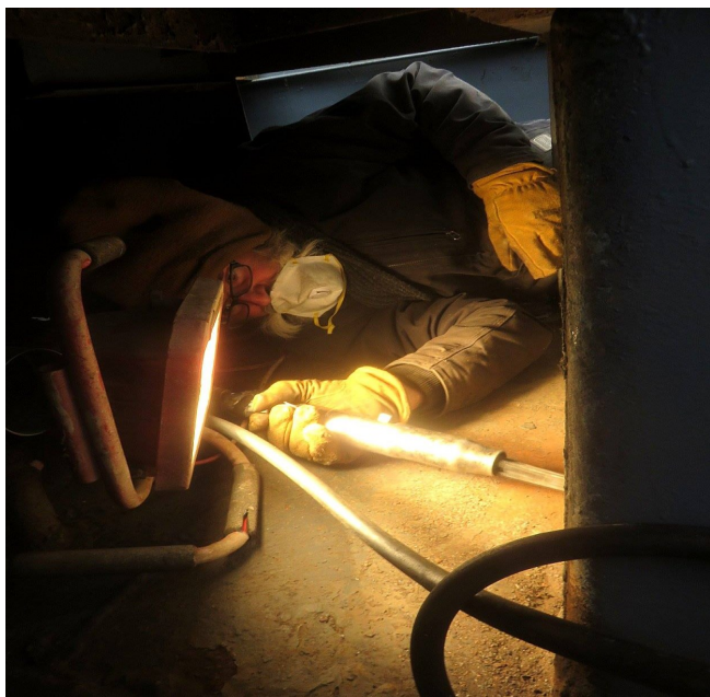
Earl Herchenroder needle scaling under the pelorus stand on the flying bridge.
