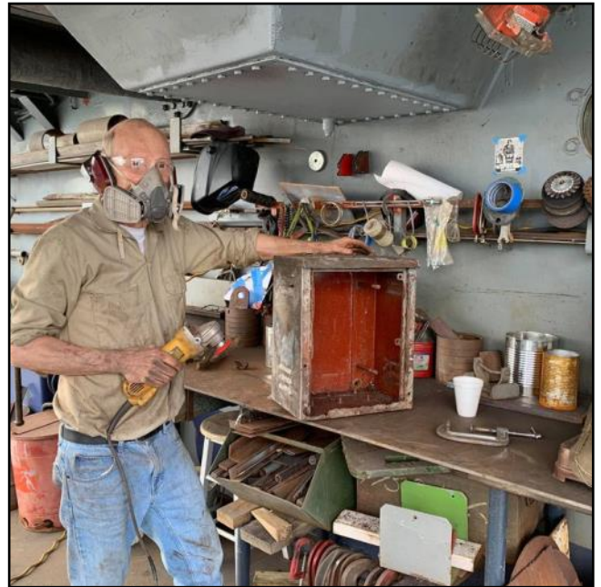
Gary restoring a motor control box.
