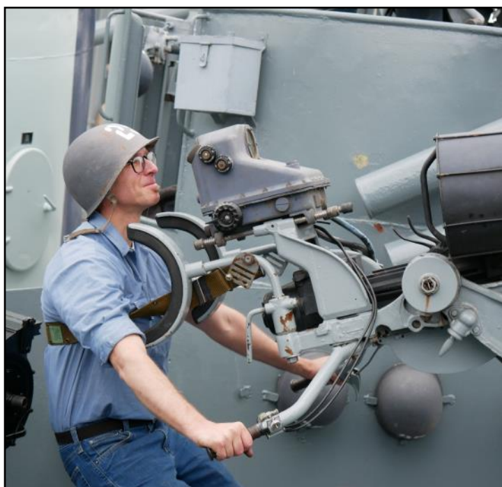
Thanks to Richard, the Mk14 gunsight is ready for displays and mounted on SLATER's 25 gun. The compressor works and the target lights.
