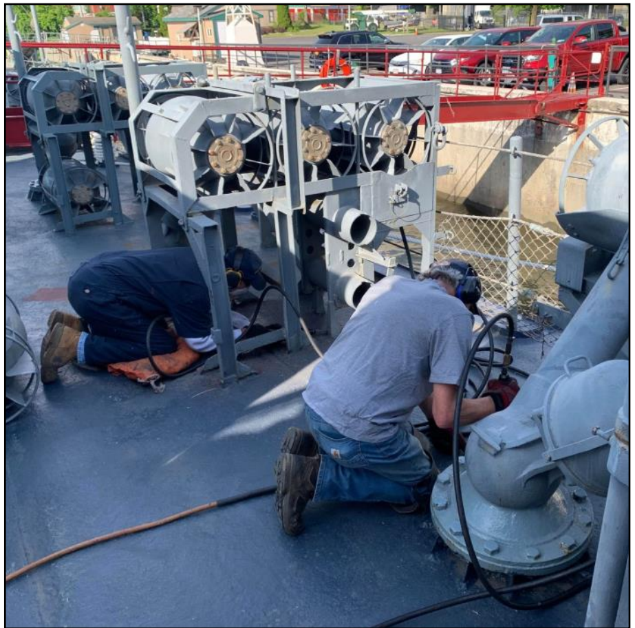
Ron Prest and Bill Wetterau are back to scaling under the roller loaders.
