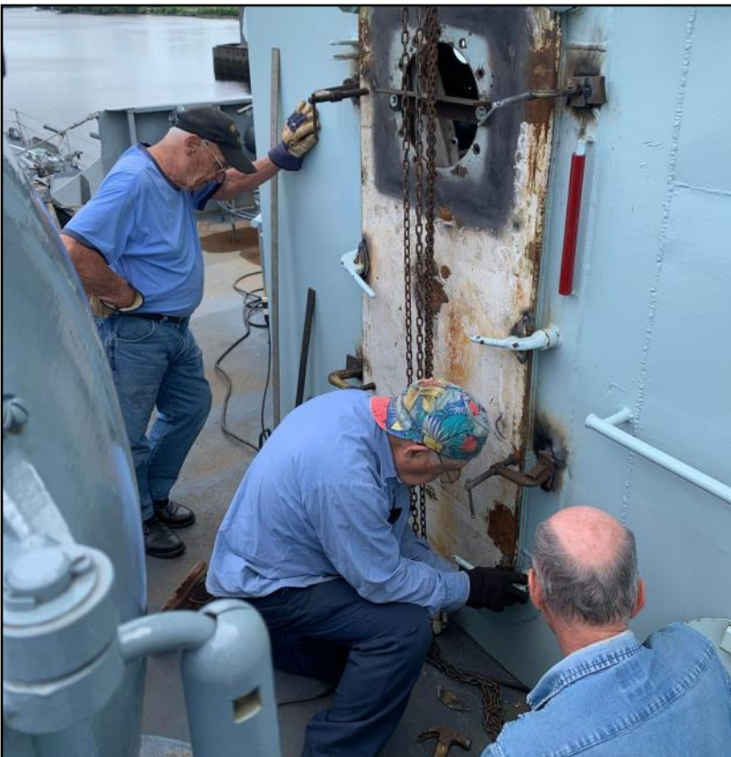
Dave, Doug, and Chuck continue work on the pilothouse watertight door.
