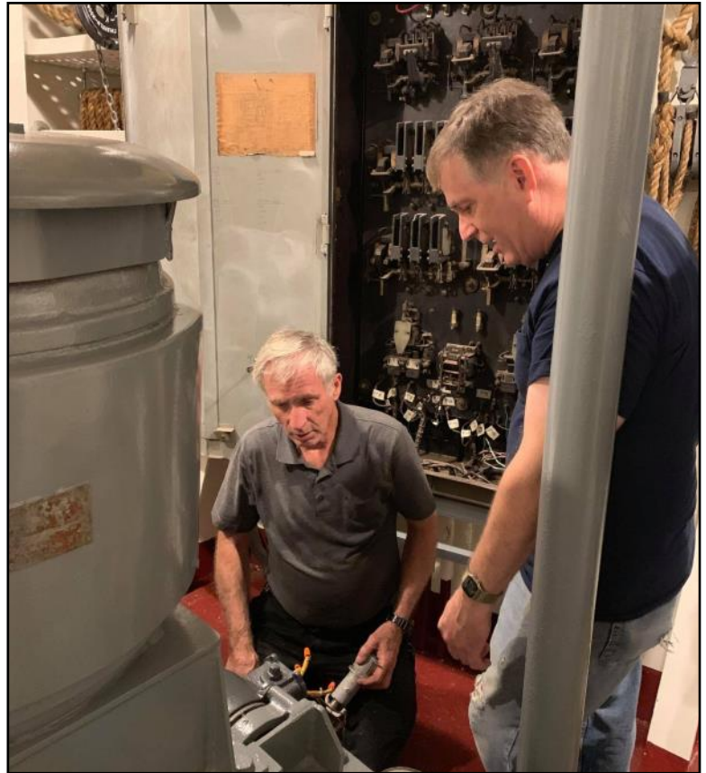
The dynamic duo, Gary and Barry, got the anchor windless electric brake working!
