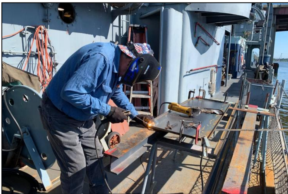
Danny is fabricating a new cover shield for the fantail 20mm ready service locker.
