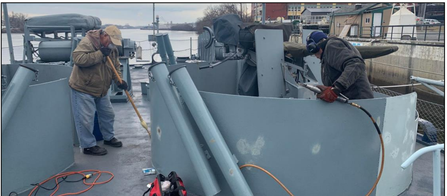
Walt Stuart, Bill Wetterau, and the deck gang have already started topside scaling and sanding to be ready for opening day.
