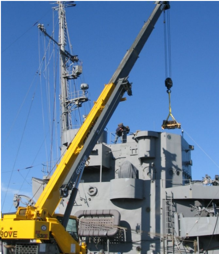
Lifting a pallet of sonar parts up to the flying bridge.
