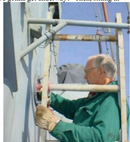
Stan Murawski purchased and is replacing all the exterior radio antenna insulators.
