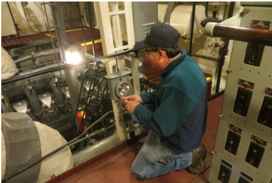
Steve Klauck checking battle lanterns as part of getting ready to re-open.
