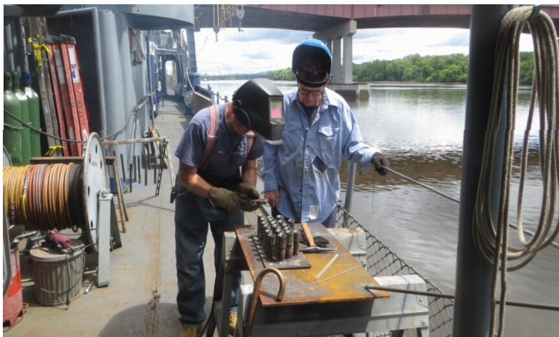
Gene Jackey and Clark Farnsworth welding up stuffing tubes.
