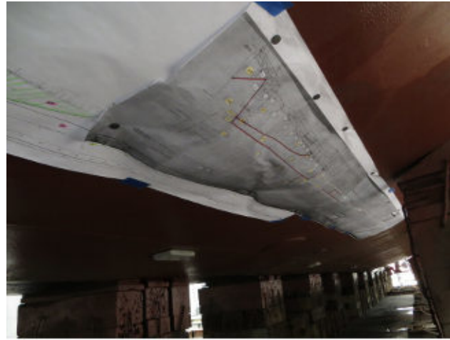
... laid out and painted the hull camouflage according to Ed Zajkowski's plans.
