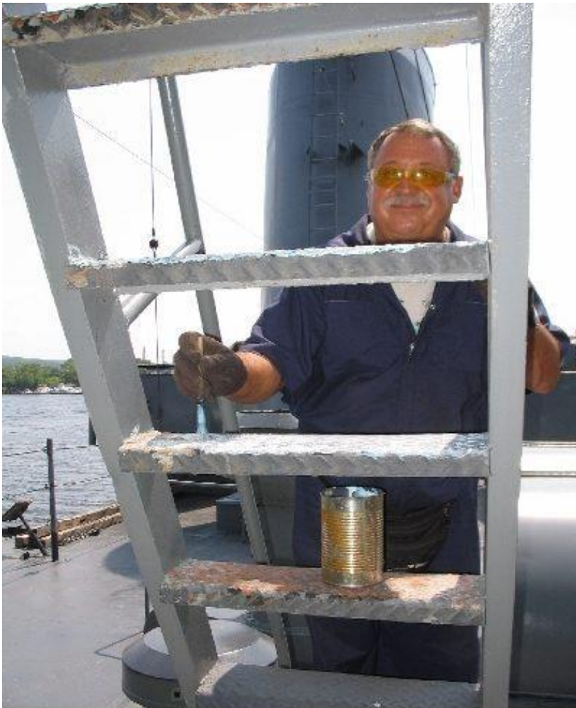
Bosun Walt Stuart renewing the non-skid on our "USS Franklin" ladder.
