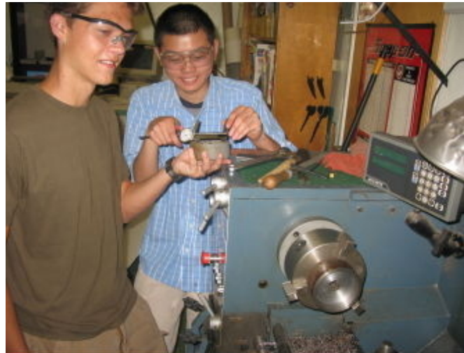
Brian Goodman and Hsin Li working with a lathe to fabricate wheels for the trolleys.
