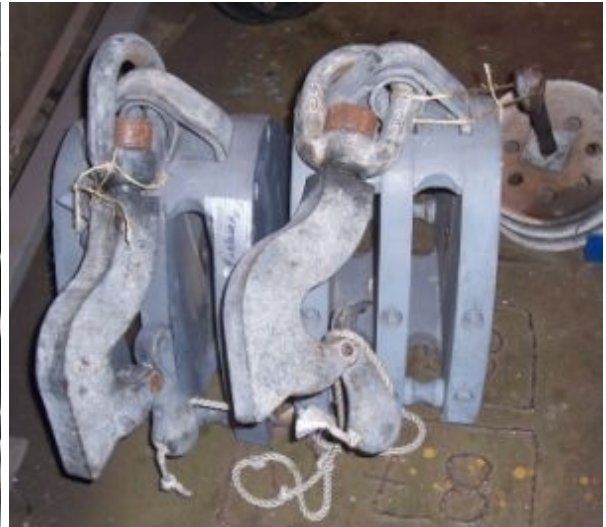
The boat fall lower blocks disassembled for inspection in the machine shop.
