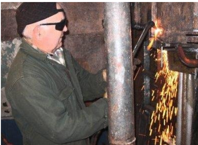
Doug Tanner has cut so much wasted metal from the forward head that the bow rose 3 feet in the water.
