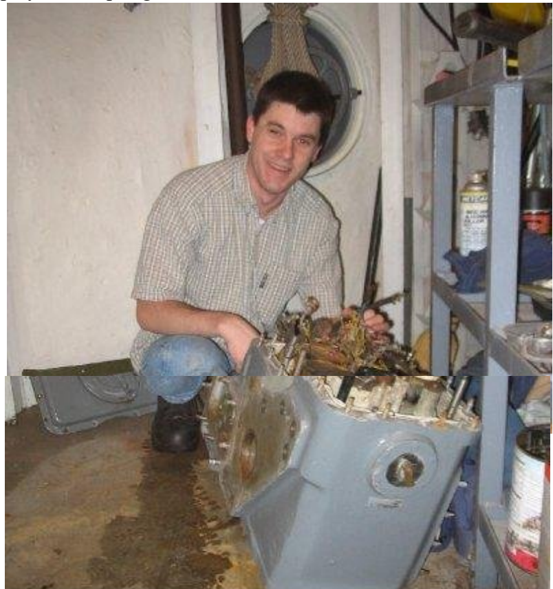
John Whalen carefully disassembles the #1 gun training mechanism to reach faulty bearings.
