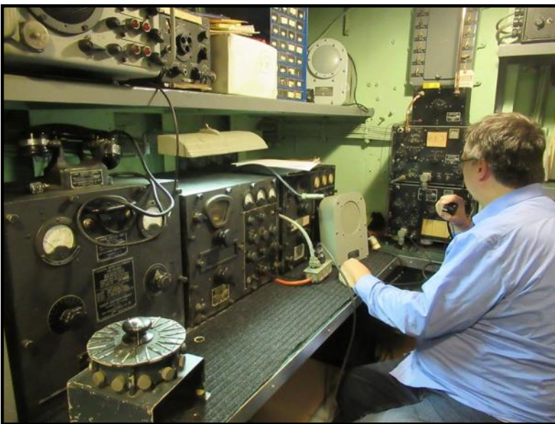
Radioman, Steve Syrotynski, completed the installation of the rebuilt RBB receiver. Here he makes a contact with the TCS transmitter.
