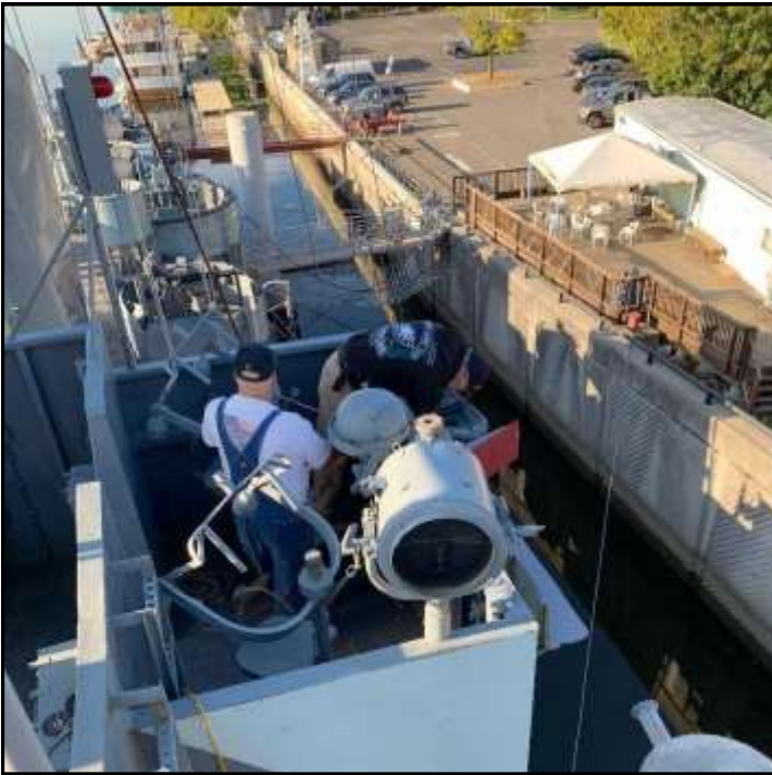
Removal of the sidelights for replacement during the fall work week.
