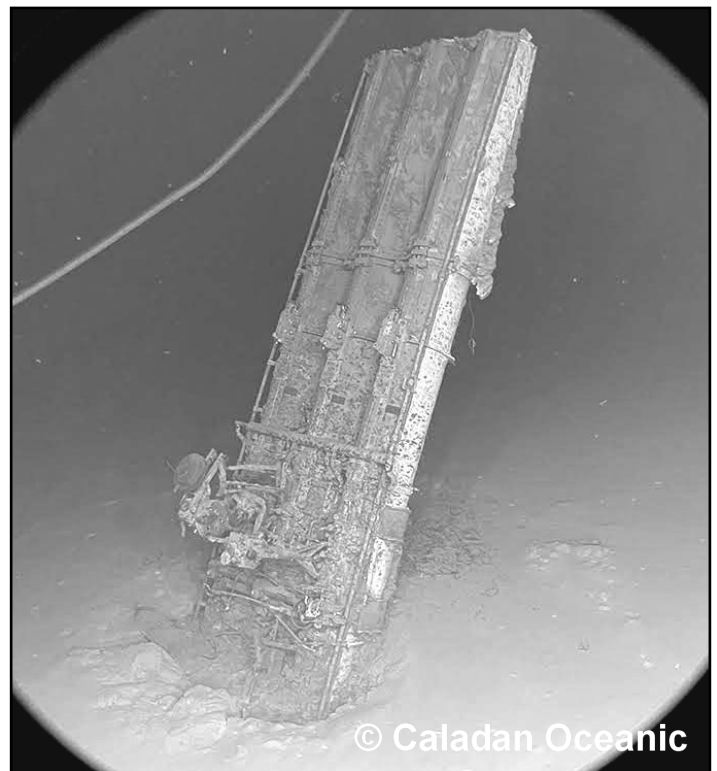
A set of triple torpedo tubes, that could only have come from one ship, USS SAMUEL B. ROBERTS. Photo courtesy of Caladan Oceanic.
