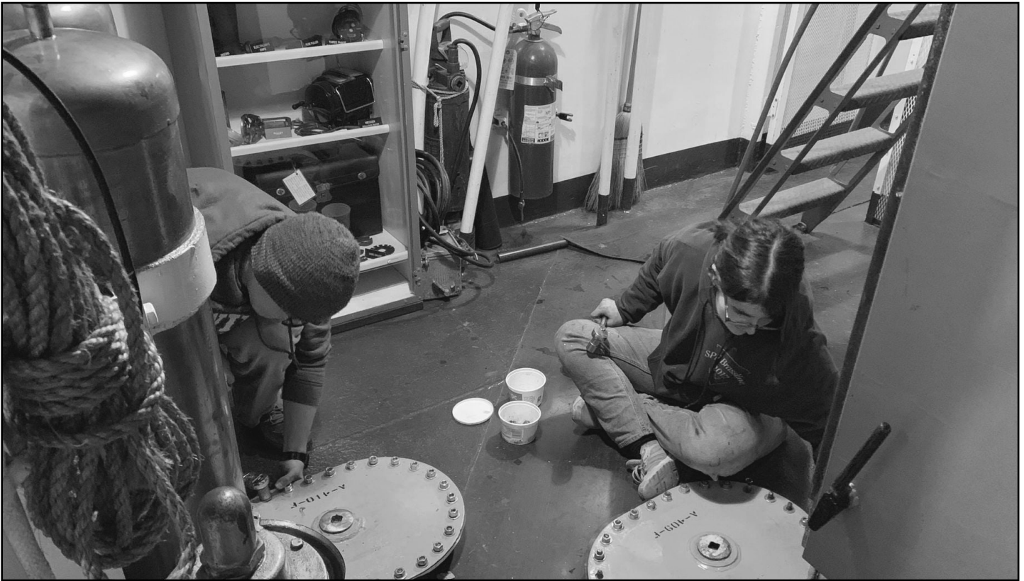
Our RPI Midshipmen play an important role. Here, they are checking the condition of our tanks and voids.
