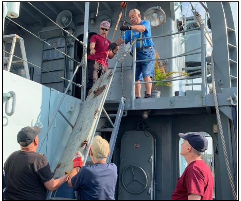
The deck gang hauls the watertight door up to the 02 level.
