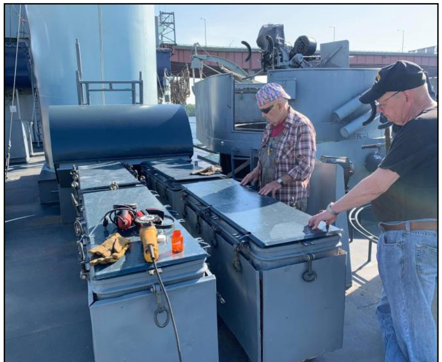
Doug and Warren check out the condition of the amidships 20mm ready service lockers.
